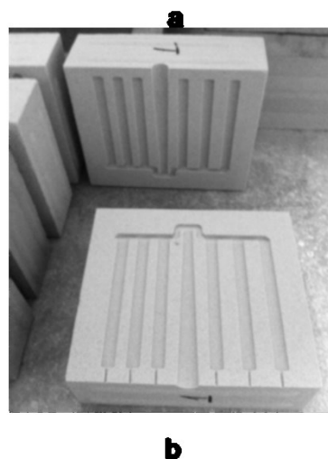
Fig. 2. a) The dimension of the mould b) Sand mould
