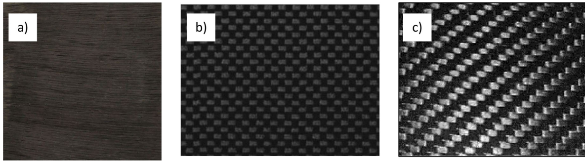
Figure 2. Test samples according to fiber orientation: (a) unidirectional (U), (b) plain weave multidirectional (P), and (c) twill 2 \times 2 weave multidirectional (T).
