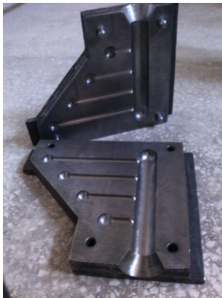
Fig. 1. The mold for the constrained rod casting (CRC) used in this study.
