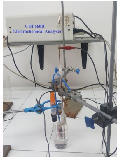
Figure 2: Three electrode cell experimental setup
