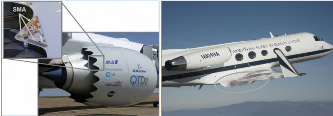
Figure 10: (a) BOEING, Variable Geometry Chevron (VGC); (b) NASA, Adaptive Compliant Trailing Edge (ACTE) project[3]
