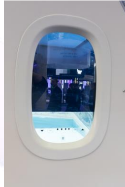
Figure 9: Electrochromic cabin window [42]
