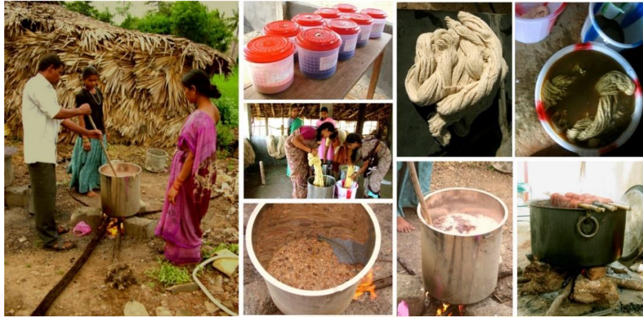
Figure 37: Dyeing of banana fibers with natural dyes [57]
