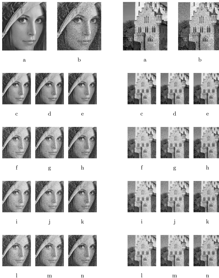
Fig. 8. MDC generation using Lena and Castle test images. (a) Part of original Image, (b) Noisy Image corrupted by the Gaussian noise of zero mean and \sigma = 0.06 , and impulse noise p = 0.06 , (c), (d), (e) Proposed Method, (f), (g), (h) GA-DWT [13], (i), (j), (k) MD-DWT [6], (l), (m), (n) MDSQ [3].
