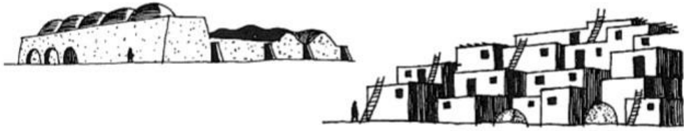
FIG. 2.4. Dwellings made of one material (mud). Left: Iran. Right: Pueblos, southwestern United States.
