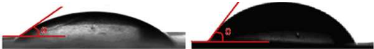
Figure 7. Contact angles measurements of the (a) NaAlg membrane (b) NaAlg-Fe 3 O 4 nanocomposites membranes
