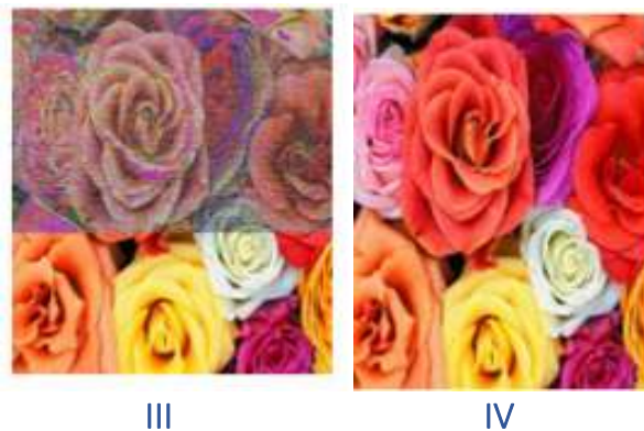
Figure 2a (rose.jpg with dimension of 560 x 448 pixels to hide the text): (III) Stego-image by means of MSB (IV) Stego-image by means of hybrid LSB-MSB
