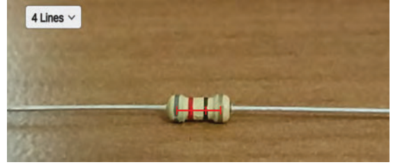
Fig. 2. Mobile application user interface with augmented horizontal line.
