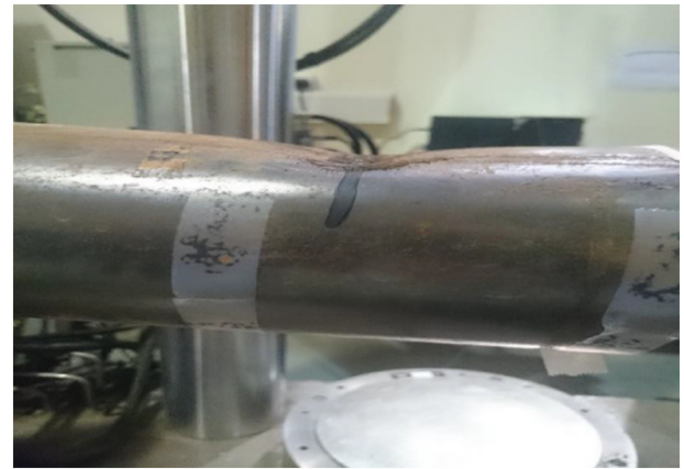
Fig. 5. Failure mode of a hollow steel tube specimen.
