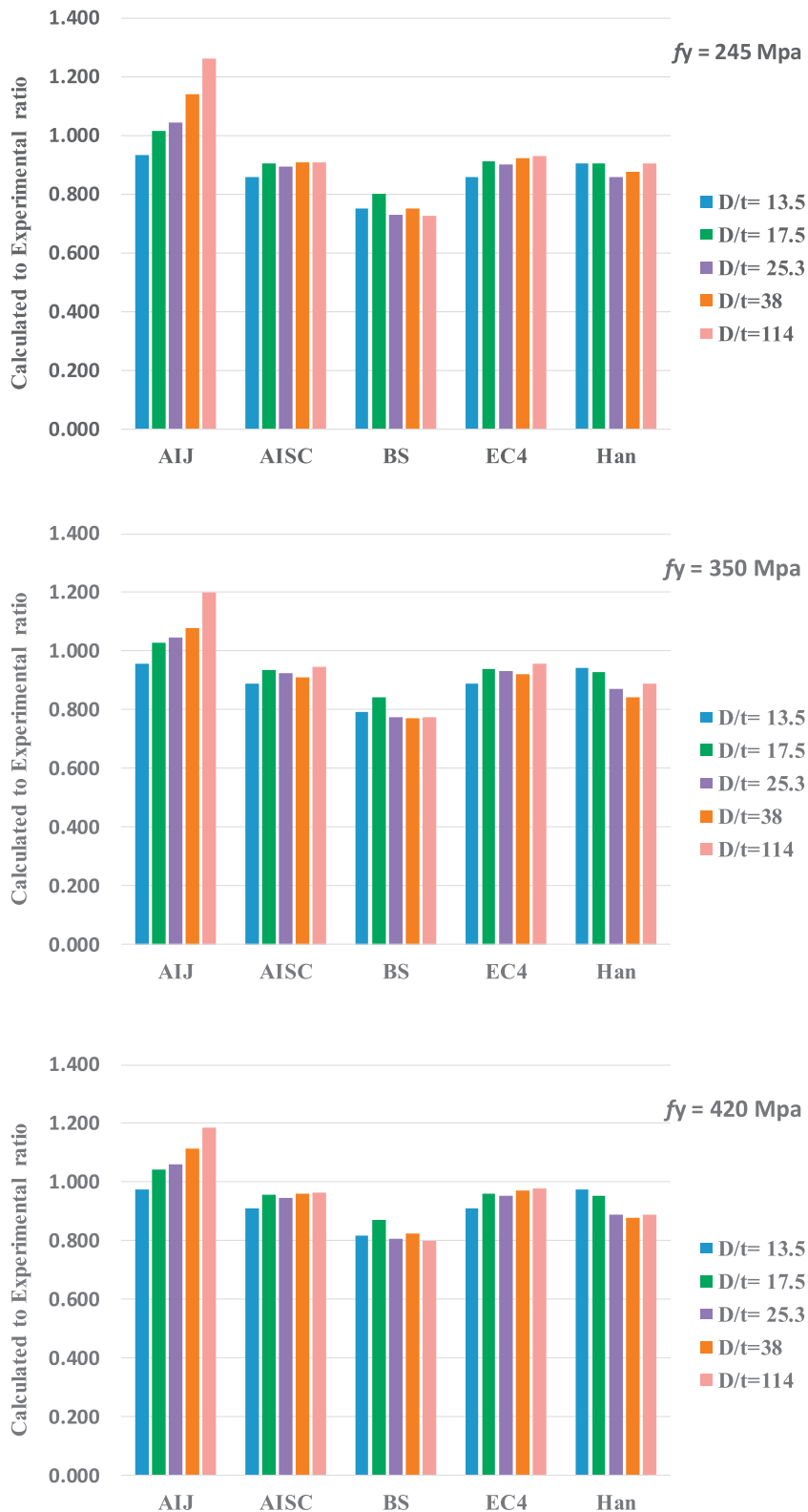
Fig. 20. Comparison between finite element results and codes equations at different D/t ratios and yield strengths.
