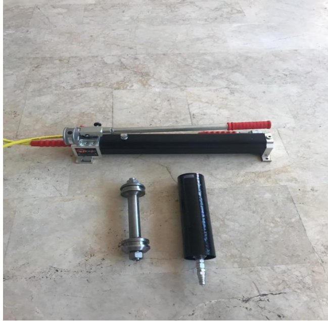
Fig.2 Pressurizing and oil filling apparatus of tubes(Yozgat, 2019)
