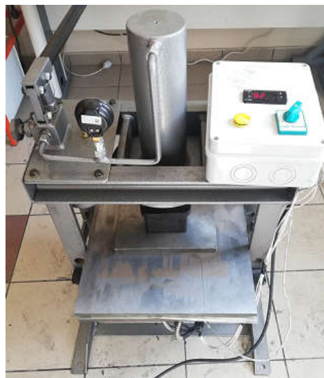
Fig. 2 The hot pressing process for produce fiber reinforced aluminum composite sandwich.
